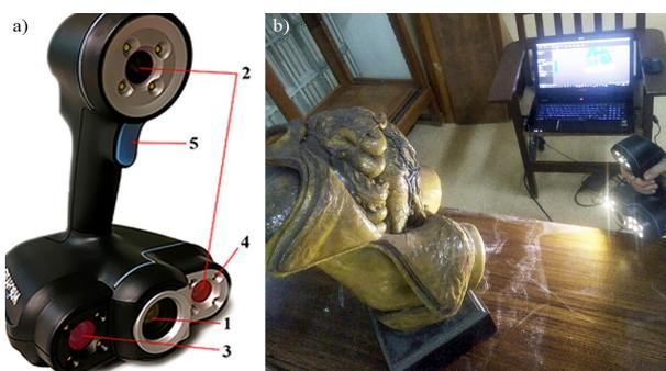
**Fig 2.** GO! SCAN50! scanner and 3D registration process. **a)** Parts of the scanner: 1. White light projector, 2. Triangulation chambers, 3. Colour camera, 4. Circular lights and 5. Trigger; **b)** 3D registration of a sculpture piece in wax at the Javier Puerta Museum of Anatomy of the Universidad Complutense of Madrid. Note how the data is collected and displayed in real time through the VXelements software.
