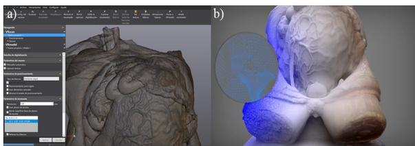
**Fig 4.** Stages of post-processing data. **a)** Mesh obtained from the point cloud corresponds to the piece under study; **b)** 3D model processed. From left to right: wireframe, neutral material, waxy material properties and colouring.
