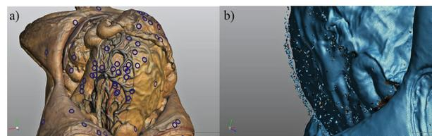
**Fig 3.** Data collection phase of the piece. **a)** Targets automatically captured by the laser scanner according to the colour variations acquired in real time; **b)** Presence of noise formed by the reverberance of laser light in contact with the smooth and shiny surface.
