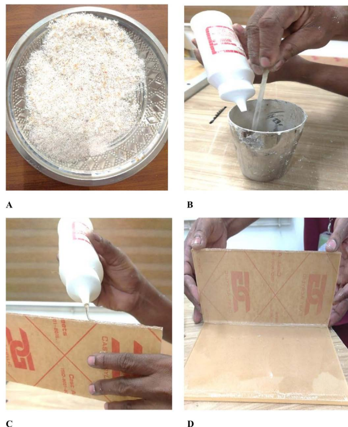
Fig. 2.- A. Acrylic scraps. B. Mixing chloroform with acrylic scraps using glass needle. C. Pouring the solvent (adhesive) along the trimmed edges of acrylic sheets. D. Joining/pasting the sheets.
