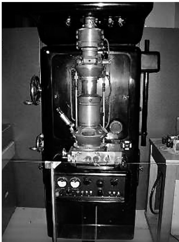
Fig. 5.- Electron microscope built by E. Ruska in 1938 and rebuilt in 1980 (Source: Wikipedia)
