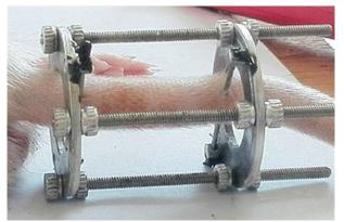
Fig 1. An Illazrov-type apparatus for rat tail segment immobilization.
